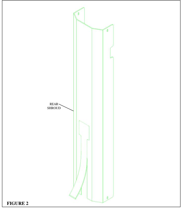
• If the 445104 SECOND STACK OPTION is not installed, the rear SHROUD opening must be removed. Apply pressure to the bottom of the SHROUD where the "V" groove is and carefuly remove the weight stack opening on the SHROUD as shown in FIGURE 2.
